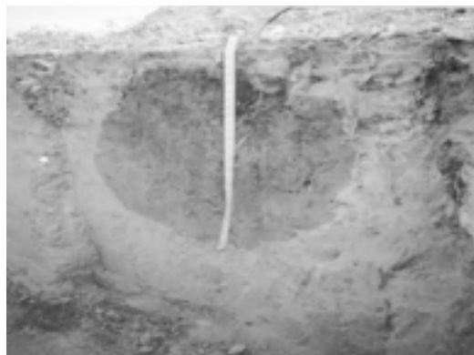
Figure 11. Position of the wetting front after 10 h irrigation applied at 1.7 l h) from simulated emitter installed at a depth of 0.30 m
